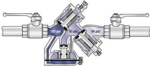
Cutaway view of a Reduced Pressure Principle (or Zone) Backflow Assembly (RPZA)
