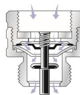
Cutaway view of a hose bib vacuum breaker
